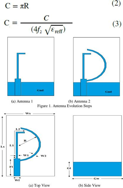
Figure 2. Geometry of the proposed dual band monopole antenna.
