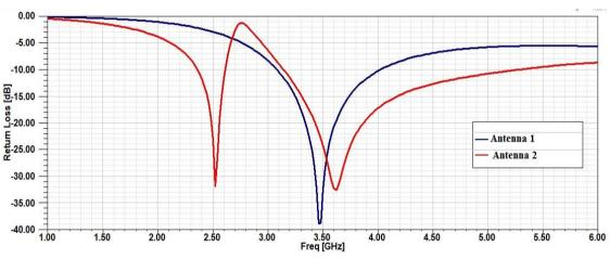
Figure 3: Simulated return loss of antenna evaluation step
