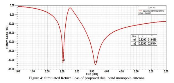
Fig.4 shows the Simulated Return Loss of proposed dual band antenna it can conclude that Return Loss value is -31.94 at 2.52GHz and is -32.53 at 3.62GHz.
